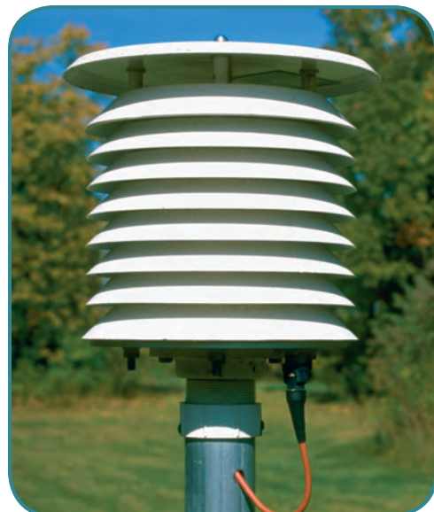
FIGURE 14 Measuring Temperature This instrument shelter contains an electrical thermometer called a thermistor.
