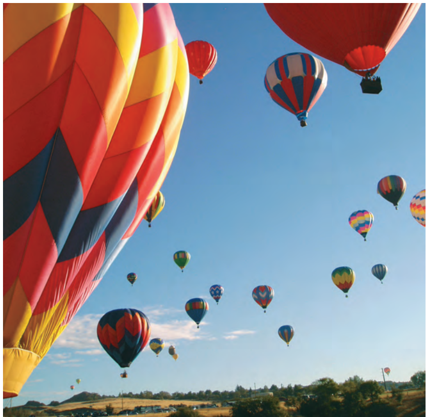
FIGURE 9 Unstable Air Hot-air balloons will rise as long as the air inside them is warmer than the air in the atmosphere surrounding them.
