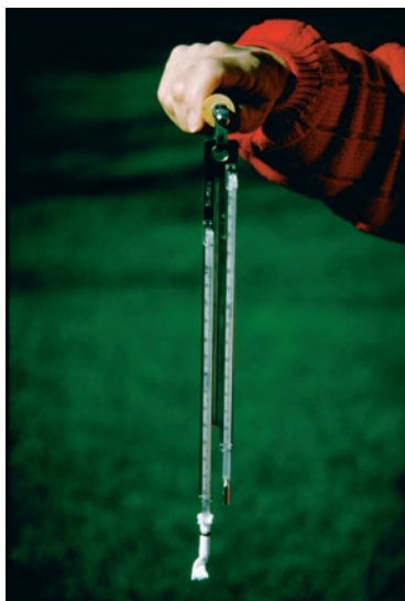
FIGURE 5 Sling Psychrometer This psychrometer is used to measure both relative humidity and dew point. Interpret Photographs Identify the wet bulb and the dry bulb in this photograph.
