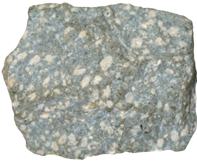
FIGURE 7 Porphyritic Texture This sample of andesite has a porphyritic texture. Note the large, light-colored crystals surrounded by darker, smaller ones. Describe How did this rock form?
