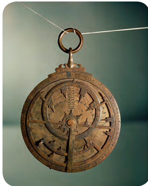
FIGURE 1 Astrolabe Early astronomers often used instruments called astrolabes to locate and predict the positions of the sun and stars.
