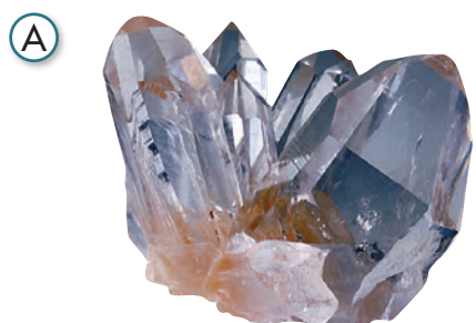
FIGURE 7 Examples of Covalent Bonds— A Quartz is a covalent compound that forms when oxygen and silicon atoms bond.
