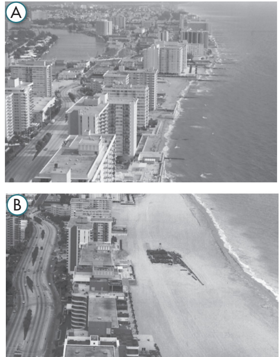
FIGURE 25 Miami Beach A Before beach nourishment B After beach nourishment Explain What are the advantages and disadvantages of beach nourishment?
