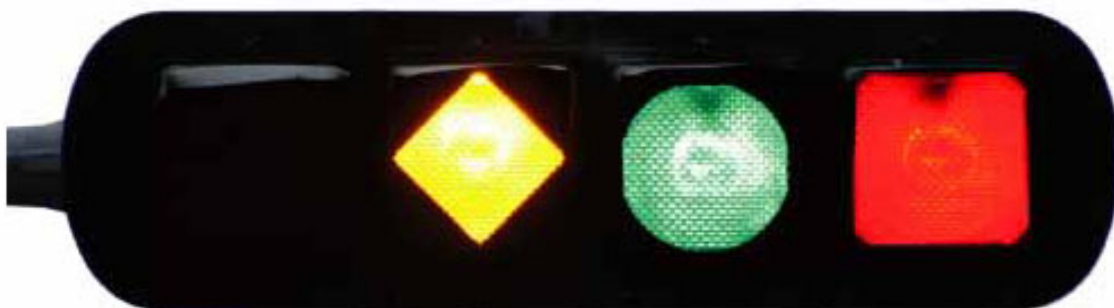
Figure 6 This stoplight in Canada is designed to help the colorblind see signals easily. This photograph was taken over a few minutes to show all three shapes.
