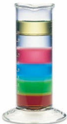
Figure 4 This graduated cylinder contains six liquids. From top to bottom, they are corn oil, water, shampoo, dish detergent, antifreeze, and maple syrup.
