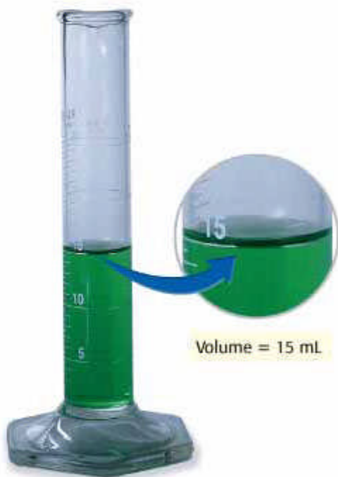
Figure 2 To measure volume correctly, read the scale of the lowest part of the meniscus (as shown) at eye level.
