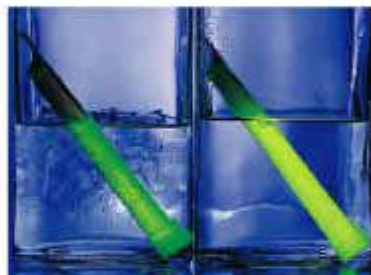
Figure 5 The light stick on the right glows brighter than the one on the left because the one on the right is warmer. The higher temperature causes the rate of the reaction to increase.
