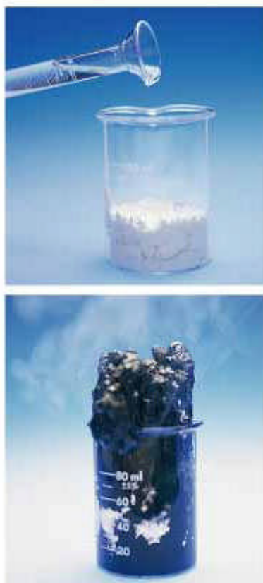
Figure 3 The top photo shows the starting substances: table sugar and sulfuric acid, a clear liquid. The substances formed in this chemical reaction are very different from the starting substances.
