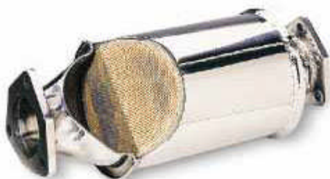
Figure 7 This catalytic converter contains platinum and palladium. These two catalysts increase the rate of reactions that make the car's exhaust less harmful.
